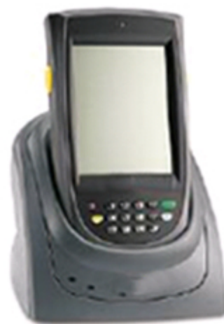
Hand Held Stock Control Device on its docking station/recharger
